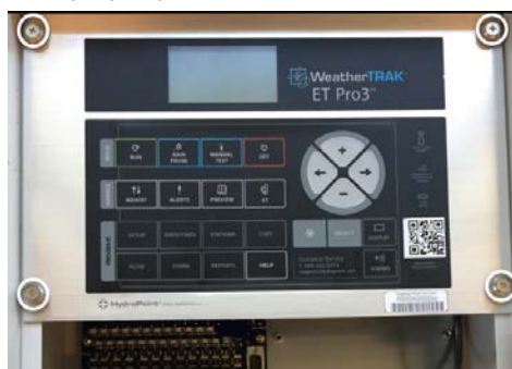
Remove 4 corner pop-up screws and flip over
