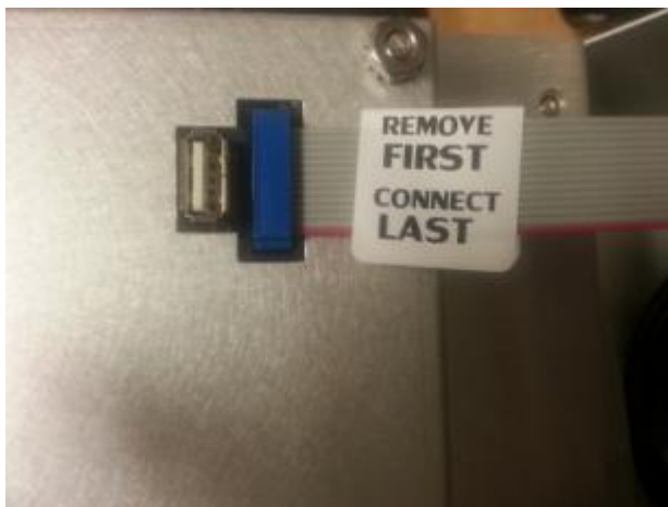
Figure 4. Command Module Ribbon Cable Connection
