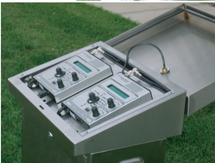
HydroPoint's WeatherTrak ET controller was part of the Irvine, Calif., Residential Reduction Study. At right is Chris Manchuck, vice president of business development for HydroPoint Data Systems, at one of the test application sites. Below is the controller system, which helped to manage water use in the test area.
